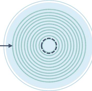
Once the center ring is dotted utilize Eyewear Inspection Job Aid to **mark the center dot by using the HD SV 0 mm seg drop**. The dotted ring is just slightly larger than the circle on the job aid so it will line up just on the inside. This center reference point is what you will use to center in the lensometer reticle for inspection.
