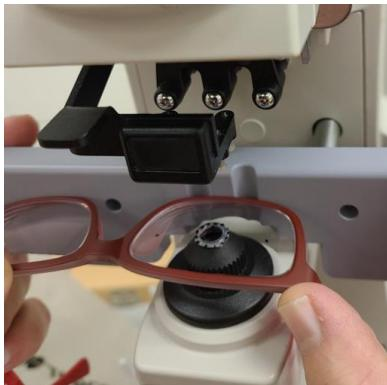
Before clamping verify with inker pen that the lens is truly centered.
